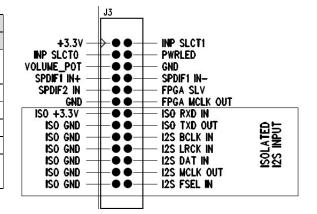
The isolated side may be powered by either 3.3V or 5V, it does not matter. In case of the DAM, it should be 3.3V taken from J3. For proper serial communication, **Pin 2** should be connected to the pin **ISO TXD OUT** and **Pin 4** to **ISO RXD IN.** Pins 3 & 5 are not used, they are there for future use.
