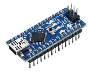
The Arduino Nano is a 5V device, so all of its pins are at 5V levels. Keep that in mind when connecting peripherals (like an SD reader). Some peripherals are designed for 3.3V logic levels.
